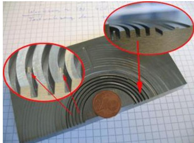
Implementation of this technology change required a lot of brainstorming e.g. in view of new tool design rules suiting milling instead of EDM operations. One must also provide for sufficient programming capacity for the creation of
