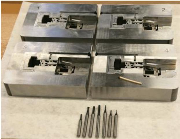
emphasize aspects such as realization time and flexibility with respect to specific demands. Many of the tools Ermet has to produce, e.g. for electronic connectors or for the embedding of metal grids, are for highly automated production. Their filigree components have to fulfil very high requirements with respect to dimensional accuracy.
